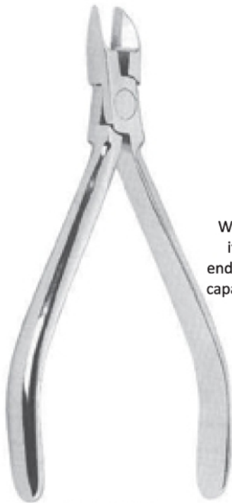
SGS 330-006 Micro-miniature light wire cutter. it cuts soft ligature wires. for use in case of limited access. Caution: maximum cutting capacity: soft ligature wire up to 0,30mm (.012")
