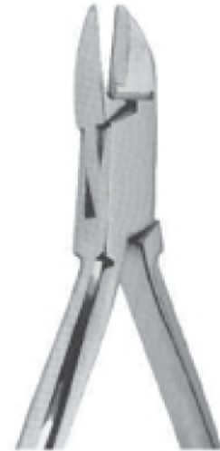
SGS 330-008 Wire cutter, for ligature wires and pins. it is strong enough to bend archwire ends after distal cutting. maximum cutting capacity up to 0,9mm (.036")
