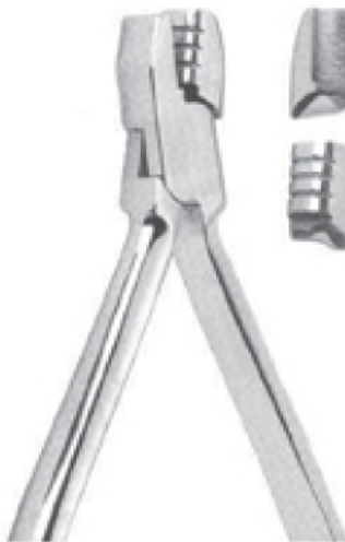
SGS 330-021 De La Rosa De La Rosa arch forming pliers. designed to form and contour arch wires on round or rectangular wire. the beaks has grooves of 0,4mm (.016") 0,46mm (.018") and 0,56mm (.022")
